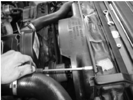
Figure 2. Remove the two 8-mm fasteners atop the fan shroud. Pull fan shroud out. Now you have more working room. (Some engines are different and may have more working room as a matter of design.)
