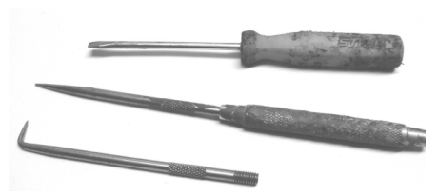
Figure B10. (a) Pry out the overhead camshaft seal with a small flat-bladed screwdriver, working diametrically opposite each pry point. Do the same for the intermediate shaft seal and crankshaft seal.
